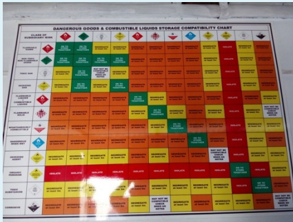
Improvement of chemical storage: Liquid storage compatibility chart in use
